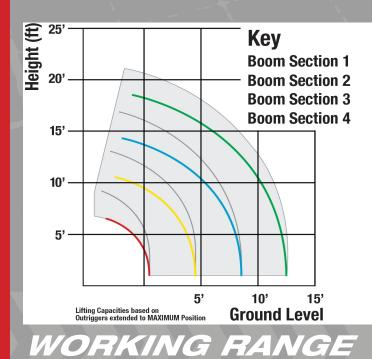
**22ft** Tip Height 1,990<sup>lbs</sup> Capacity **48V** Battery Power
